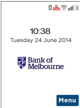
The terminal display shows information such as the battery strength, connection strength, date and time.
